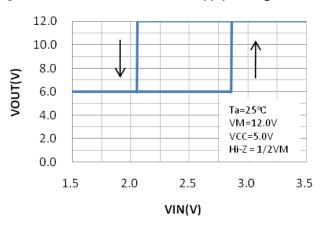
Figure 5. Output voltage vs. Input voltage
