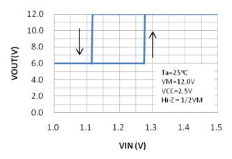
Figure 4. Output voltage vs. Input voltage
