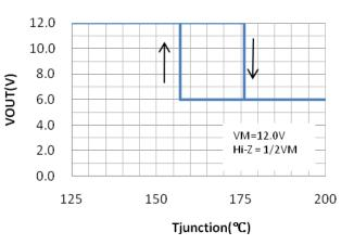
Figure 15. Thermal shutdown characteristic
