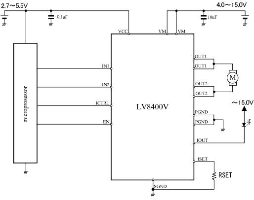
Figure 17. Sample Application Circuit
