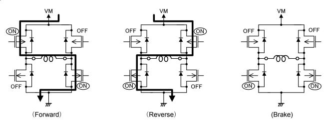
Figure 16. Output stage transistor function
