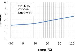
Figure 13. IOUT on-resistance vs. Temperature
