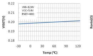
Figure 12. VISET voltage vs. Temperature
