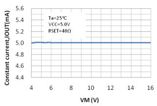
Figure 11. Constant current, IOUT vs. VM supply voltage
