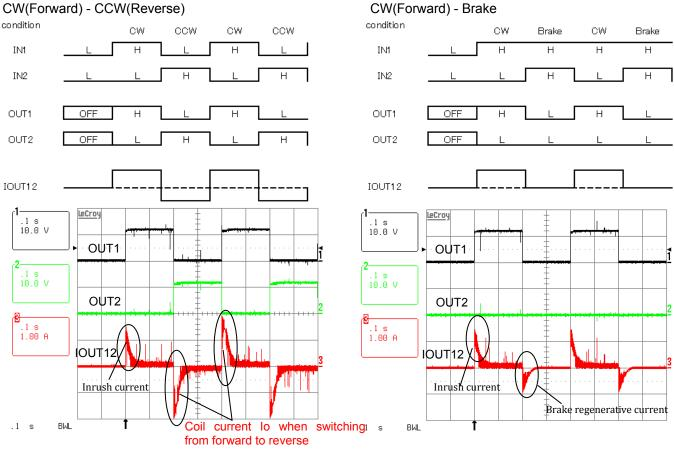
Figure 18. Driving waveform of DC motor
