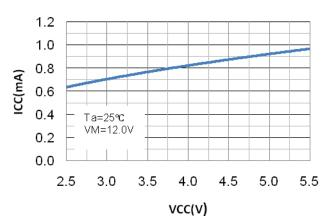
Figure 3. VCC current drain vs. VCC supply voltage
