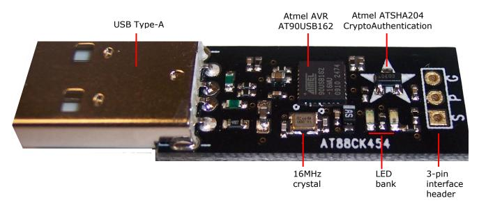
Figure 1-2. Bottom side components placement
